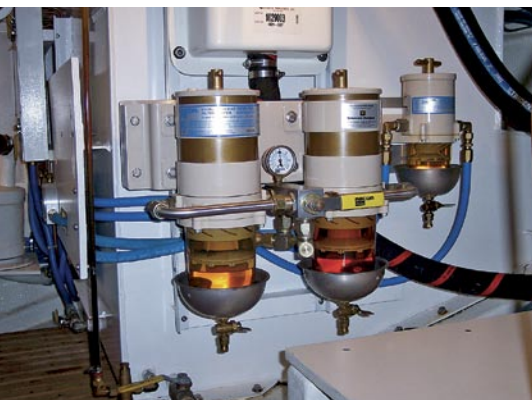
The writer's Grand Banks 42 uses Racor 75/900MAX primary fuel filter/water separators with one-handle valve control allowing isolation of one filter at a time for servicing, even during engine operation. The vacuum/pressure gauge indicates when the filter needs to be serviced, and the valves permit easy draining of water and contaminants from the separator bowl.
