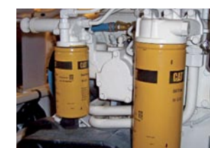
Maramor's Caterpillar 2-micron engine-mounted secondary fuel filter, left (oil filter, right) and fuel priming pump are mounted on the front of the engine for easy access. The only tool needed for a filter change is a strap wrench.
